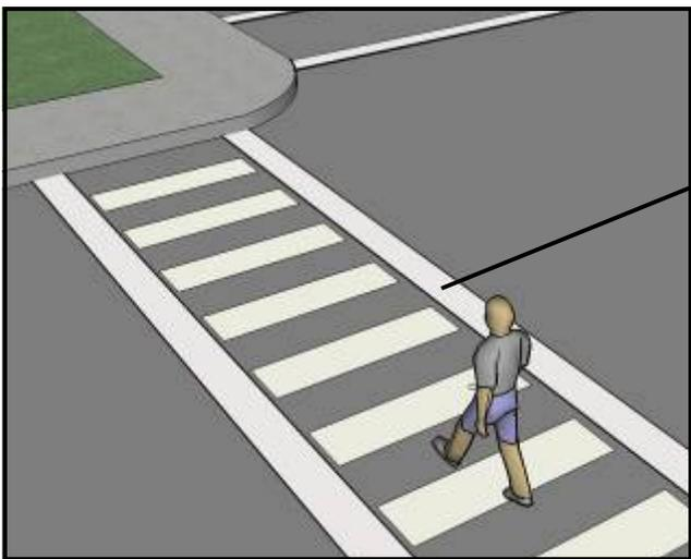
If line markings such as ladder stripes are present it is most likely that the pavement will have to be removed and replaced. These heavy markings cannot be removed from the surface without leaving unsightly marks (ghost lines).
